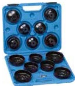
Misure (ø mm - lati) 65 mm - 14, 65/67 mm - 14, 68 mm - 14, 74 mm - 15, 74/76 mm - 15, 75/77 mm - 15, 76 mm - 14, 76 mm - 30, 80 mm - 15, 80/82 mm - 15, 90 mm - 15, 93 mm - 15, 93 mm - 36, 100 mm - 15
