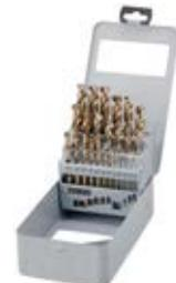
**P064/19A****SERIE PUNTE AL COBALTO**AUTOCENTRANTI, DESTRE, SERIE CORTA, RETTIFICATE, PER LAVORAZIONE DI MATERIALI CON RESISTENZA R= 1400 N/mm<sup>2</sup>, DUREZZA PUNTA HV= 850 ÷ 900
